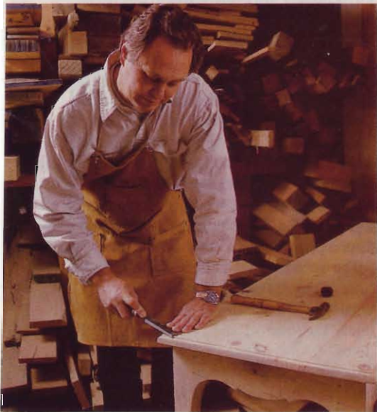
With a chisel, Greg shaves off small areas of a cypress table's machined edge. Finished, it will look centuries old.
